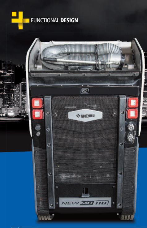
The power of this new compact sweeper is hinted at by the many features fully integrated on the rear face, such as the square LED lights, the water filling and cleaning functions and the wanderhose located in the rear door compartment.
