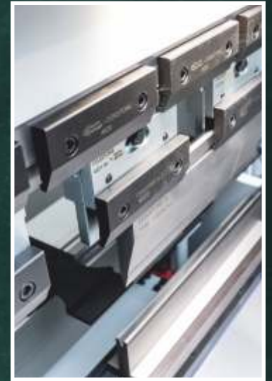
Promecam tooling (European style tooling).
