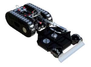
"CLIIN Robotics' innovative Robotic Antifouling system seamlessly operates above and below the waterline, even with strong currents. It efficiently removes marine biofouling from light slime to heavy animal fouling, optimizing sustainable hull performance while minimizing fuel consumption and operational costs."
