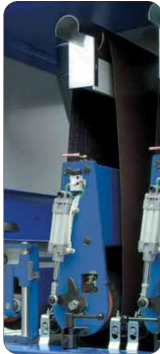
Cylinder unit equipped with 6 position Grit-set selector, revolver-type, for easily switching abrasive grit sequence, pneumatically activated.
