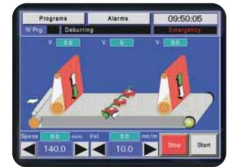
The PLC panel VISION (optional) enables the visualization in a touch-screen monitor of the actual setup data and operation of the machine, and to store many complete working programmes.
