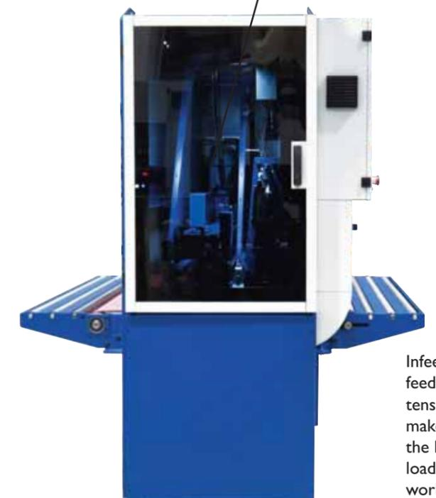
Infeed and outfeed table extensions to make easier the loading-unloading of workpieces.
