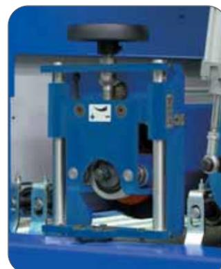
Longitudinal brush unit Ø 180 mm with manual height adjustment and mechanical thickness read-out. Lateral oscillation system of brush. Our brushes are available in various materials: steel, stainless steel, scotch brite and many others.
