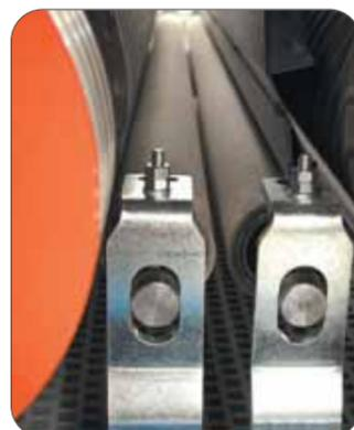
Double pressure rollers with micrometric precision adjustment mounted in front and rear of each working unit.
