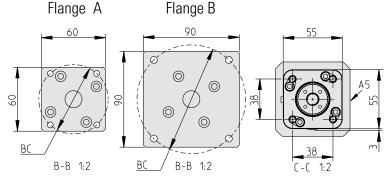
A1: grease port A2: M6 thread, max. depth 30 mm A3: no thread A4: male threaded rod end shown, see ordering key and accessories for information on all available ends. A5: side of cover tube for mounting of sensors. A6: distance to center of coupling tightening hole.
