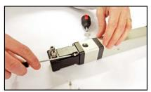
Tighten motor mounting screws
