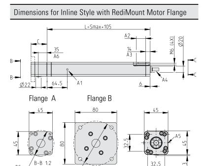
A1: grease port A2: M6 thread, max. depth 30 mm A3: no thread A4: male threaded rod end shown, see ordering key and accessories for information on all available ends. A5: side of cover tube for mounting of sensors. A6: distance to center of coupling tightening hole.
