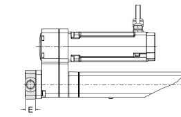
The fixed front and rear trunnions consist of a plate with two shafts and come mounted from the factory if the ordering code states that the unit shall be equipped with one. They can also be ordered as a separate parts (all necessary actuator attachment screws are included) using the part numbers. The rear trunnion can only be mounted on to the belt gear on parallel style actuators.
