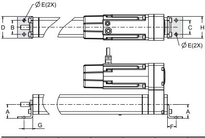
The foot mount consists of a front and rear bracket and comes mounted from the factory if the ordering code states that the unit shall be equipped with one. It can also be ordered as a separate part (all necessary actuator attachment screws are included) using the part number.
