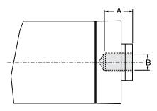
The female threaded rod end comes mounted from the factory if the ordering code states that the unit shall be equipped with one.
