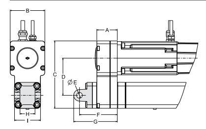
The rear clevis consists of a bracket and comes mounted from the factory if the ordering code states that the unit shall be equipped with one. It can also be ordered as a separate part using the part number in which case it is delivered with the necessary screws to attach it to the actuator.
