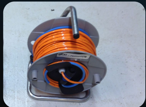
Control cable for remote operation of the Abrajet machine
