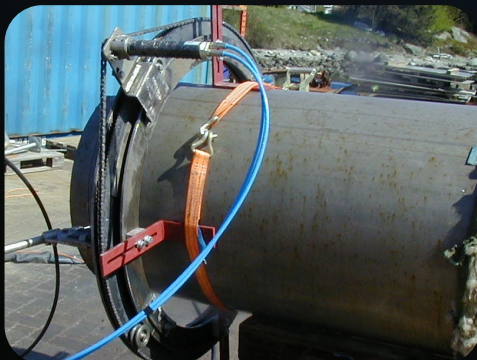
Clamp pipe cutter for particularly precise cuts.
