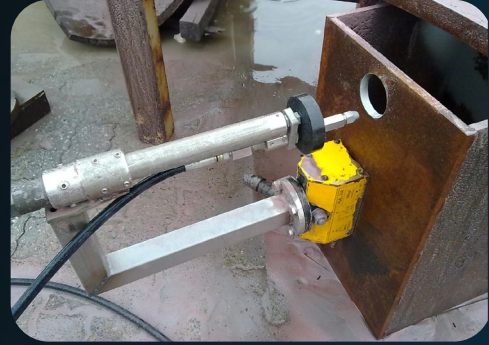
Cutting unit for cutting holes with pneumatic operation and stepless adjustment. Diameter of 200 mm - 1200 mm..
