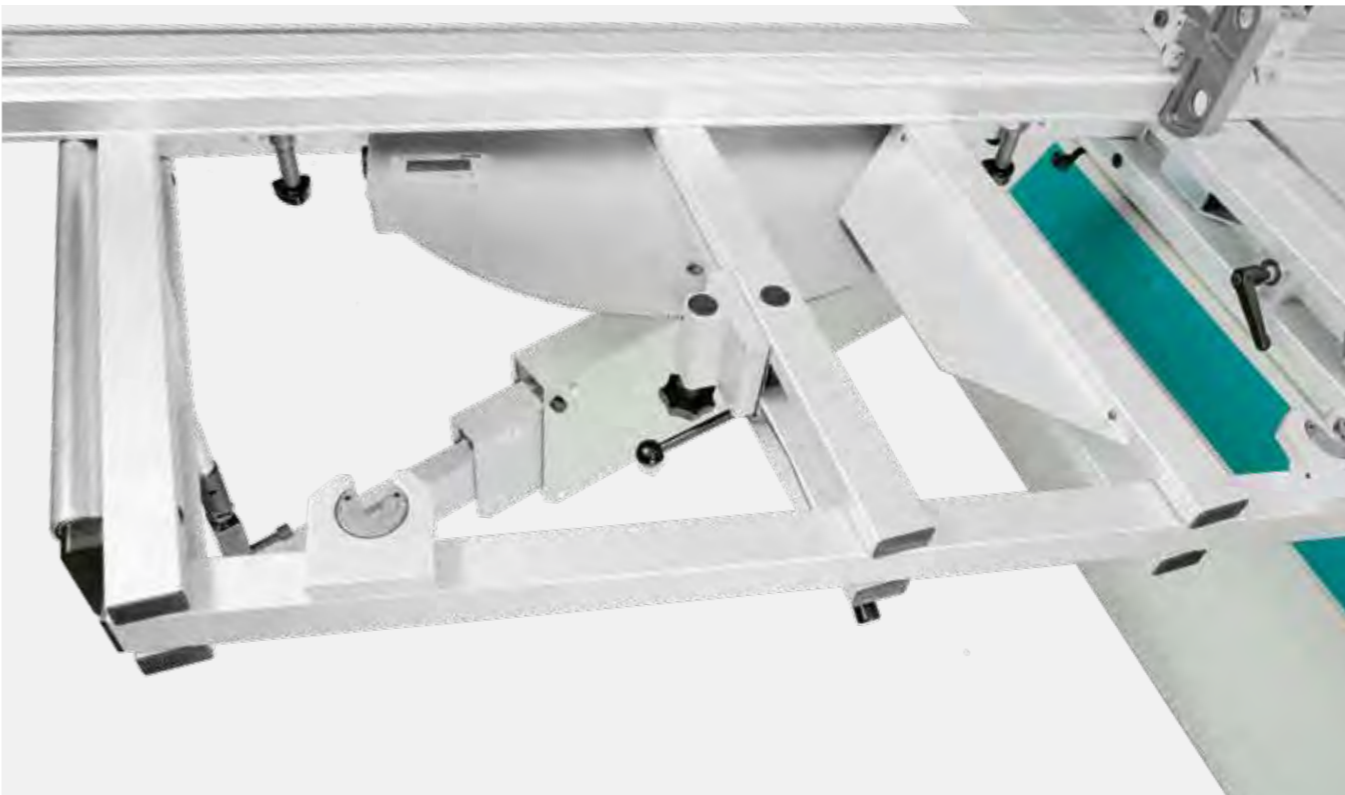
Fine adjustment, clamping mechanism and digital display of mitre cross-cut table | Txx65
