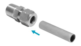
1. Insert prepared tubing into Hy-Lok tube fittings until tubing end is firmly seated the shoulder of the fitting body and make sure that the nut is finger-tight.
