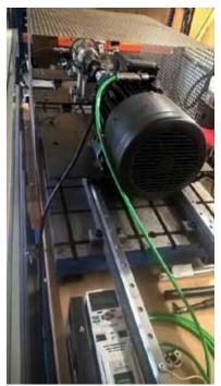
Test machine up to 150Nm.
