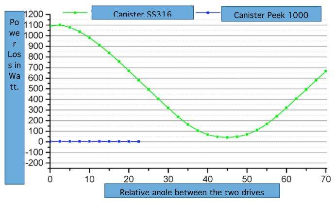
The table above shows the power loss at 1800 RPM with non-slip and under maximum work load.
