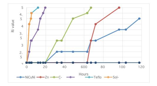
Figure 4 – Salt spray test of the samples graded according to ISO 4628-3:2003.
