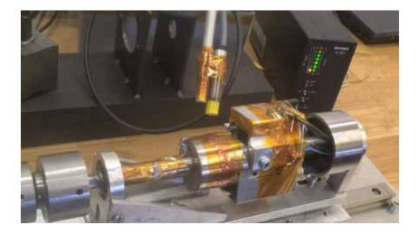
Test unit for testing our coupling for 0.001-10Nm.
