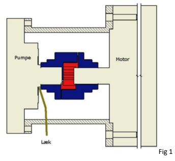
A magnetic coupling system is a good solusion when you want to avoid oil leakage. We can use a Canister, cf. Fig. 2, combined with an O-ring or a flat seal to avoid leakage. In some cases, it can also be used to prevent toxic liquid and gas release into the air, and then have an Ex approved solution. (Directive 94/9/EC (replaced by 2014/34/EU from 20 April 2016)
