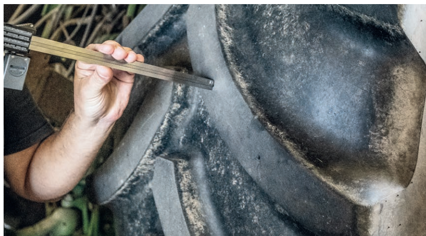
Figure 3: Wear measurement with depth stop
