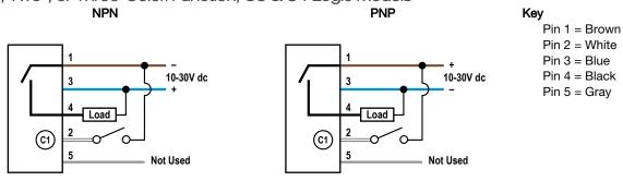
Cabled wiring diagrams are shown. Quick disconnect wiring diagrams are functionally identical.
