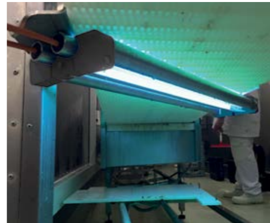
The sterilAir® T2018 is mounted under the conveyor belt using a two-point screw connection. The system can be optimally adapted to the various belt widths by inclined installation.
