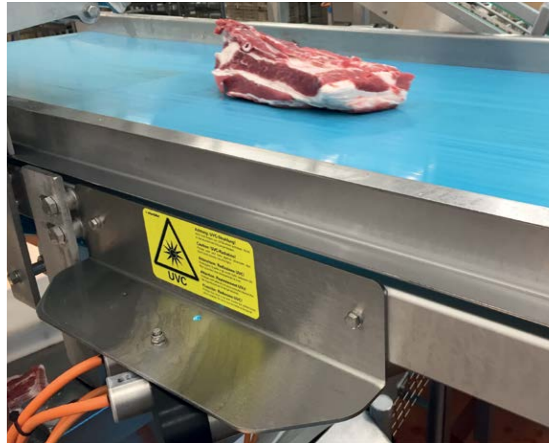
The sterilAir® T2018 is mounted under the conveyor belt using a two-point screw connection. The system can be optimally adapted to the various belt widths by inclined installation.
