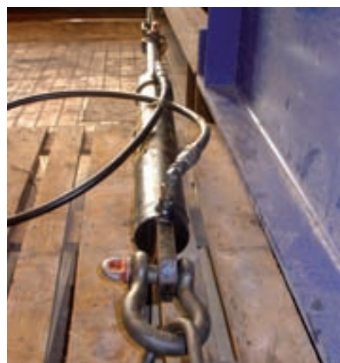
Hydraulic pulling cylinder offering great precision and strength.
