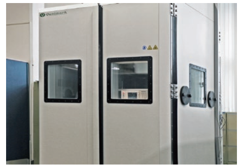
Highly Accelerated Life Testing Equipment
