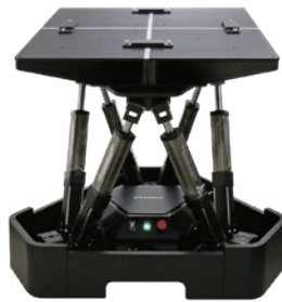
6-axis WPT test platform
