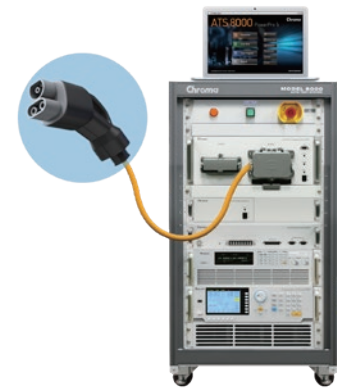
EV AC/DC charging EOL ATS
