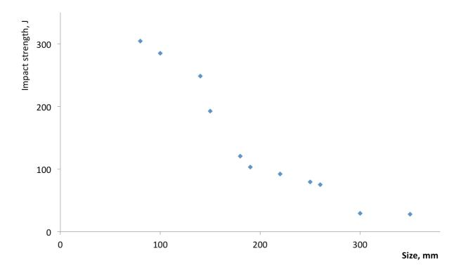
Figure 2. Typical impact energy values for Sandvik SAF 32760 in different sizes at -46°C (-50°F), using standard Charpy V specimens.
