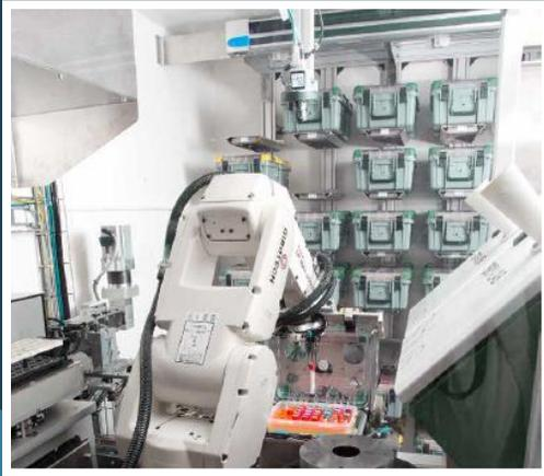
GIBOSORT is an automated solution for handling blood- or other biological samples. It automatically unpacks and empties all commonly used bio sample transport containers and forwards their content via pneumatic delivery, conveyor, postage crates or other means.
