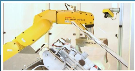
The solution's task is to separate and sort the medicaments as well as reading the barcodes, and then deliver the products to Apostore's internal storage system together with barcodes, thereby obtaining full-automatic storage. When delivering to the storage system it ensures that the products are positioned correctly on the way to the storage robot. The medicine robot handles both square and round seals, glass, cardboard and plastic packaging.
