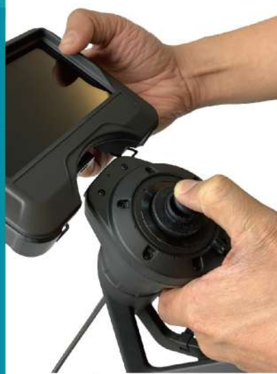
Interchangeable Probes (3.9mm/6.0mm)
