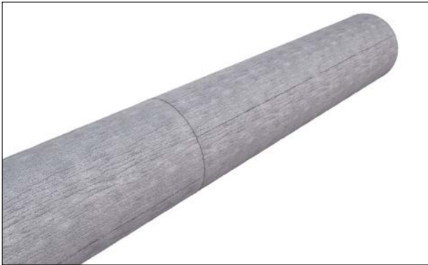
Figure 10: Circumferential and longitudinal seams are tightly butted
