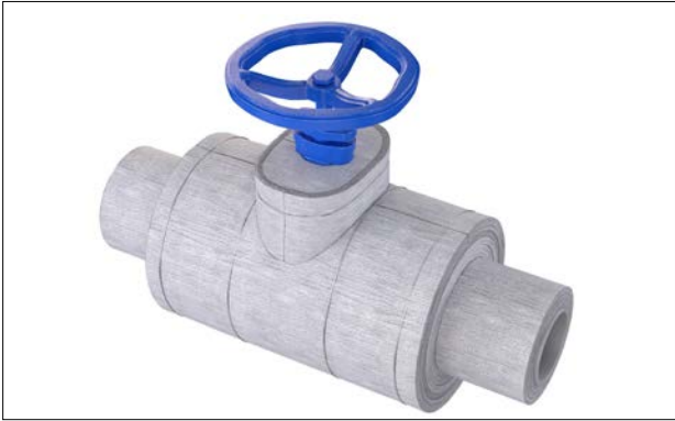
Figure 63: Installing spindle bonnet tee fitting cover.
