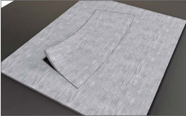
Figure 46: Cutting of reducer pattern.
