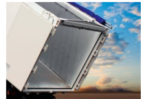
Lock the wing doors to the sides to load or unload packaged goods.
