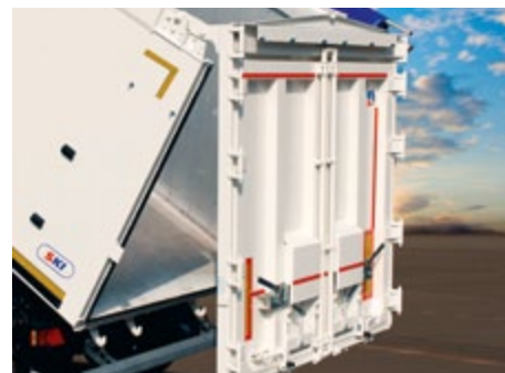
The combi-door with a pendulum frame and roof bow as a pendulum tailgate for partial unloading.
