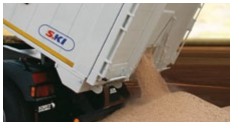
The grain slider enables the easy and controlled unloading of fine-grain crops.
