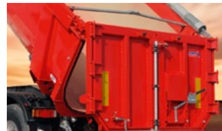
The wing door possesses a pendulum frame. This allows it to open like a pendulum tailgate.
