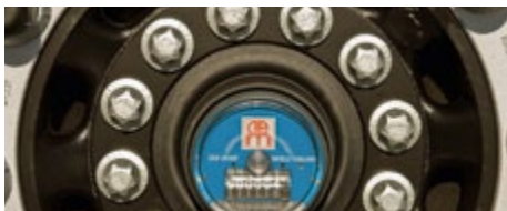
The odometer mounted on the wheel hub provides reliable information about your tipper trailer's mileage.
