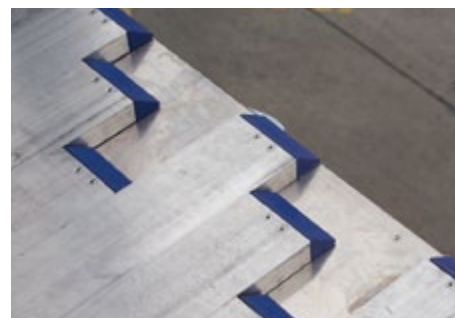
Hydraulically powered aluminium sliding floor profiles move the load.
