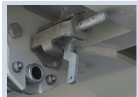
When using the grain slider to unload the trailer, pegs block the hook lock.
