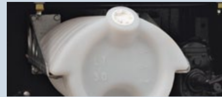
The water tank mounted on the I-beam can hold 30 litres.
