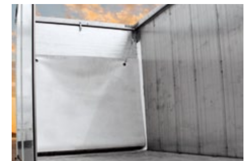
A moving wall ensures that fine-grain bulk goods are completely unloaded.
