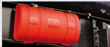
The fire extinguisher is located in a protected location on the frame and rapidly accessible in the event of an emergency.
