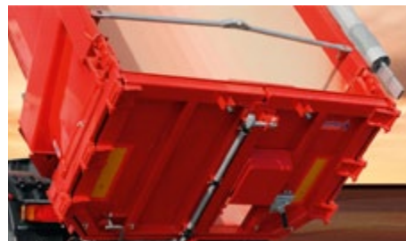
Opening the grain slider in the combi-door enables precise quantities to be unloaded.
