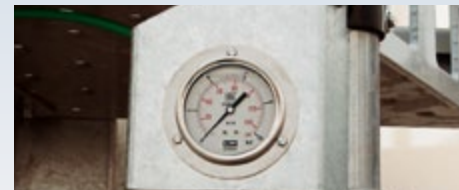
The loading pressure gauge for the air bellows pressure can be used to prevent overloading and to calculate the payload.
