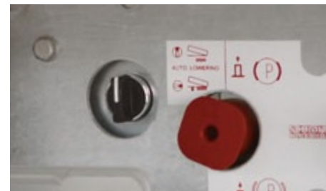
The automatic lowering function provides greater stability when tipping.
