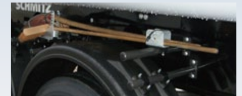
Conveniently mounted on the I-beam: The brush and shovel are easily accessible and rapidly stowed.
