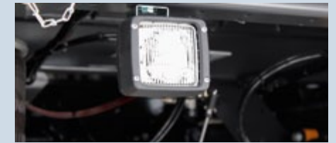
The spotlight on the rear cross-member illuminates the area behind the body for increased safety.
