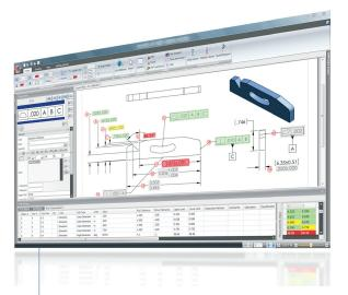
Characteristics are automatically highlighted in green, red, or yellow to instantly show which are in tolerance, out of tolerance, or marginally within tolerance.
