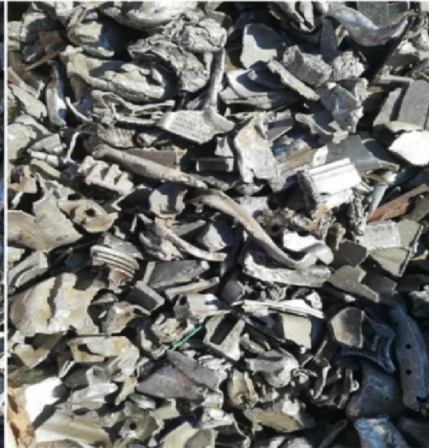
Pass 2 – Negative Output Heavy aluminum alloys
