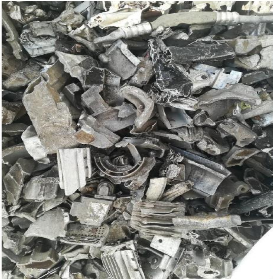
Pass 3 – Positive Output Low quality aluminium (with inclusion)
