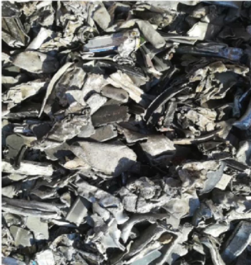
Pass 2 – Positive Output Light aluminum alloys
