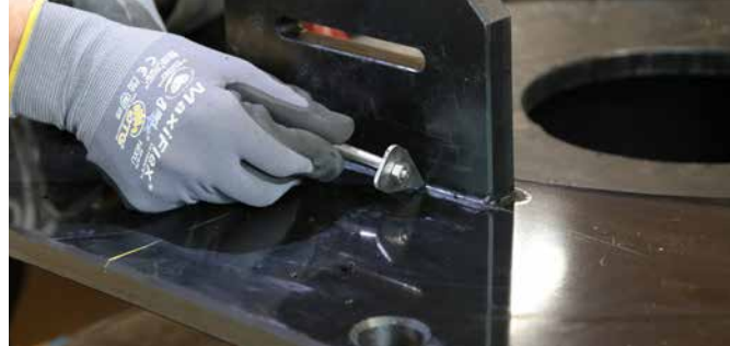
With the contour scraper, perfect weld seam pre- and post-processing is achieved
