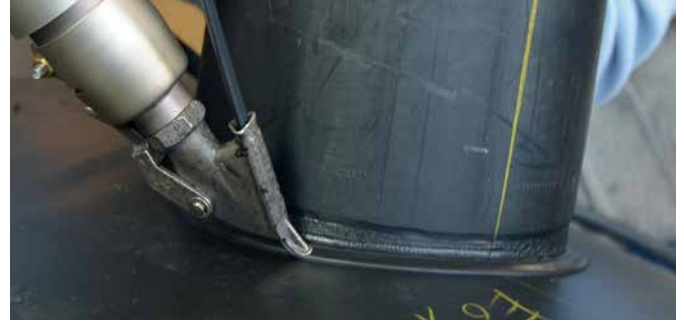
Draw welding with combination nozzle
