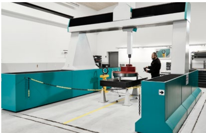
Specially designed building adapted for measurement technology including vibration-free foundation.
