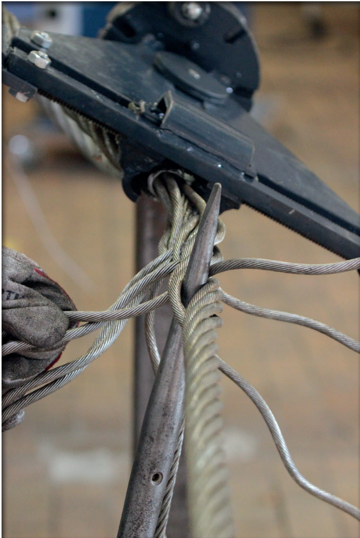
Hand splicing of a steel wire rope
