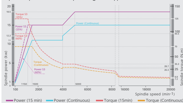
Spindle power and torque diagram (Type: aiLL 8/20000)
