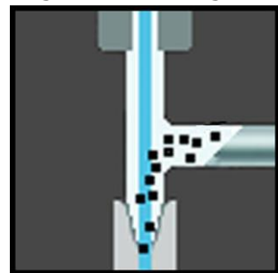
Fig. 2 Abrasive medlet sugas in i jetstrålen
