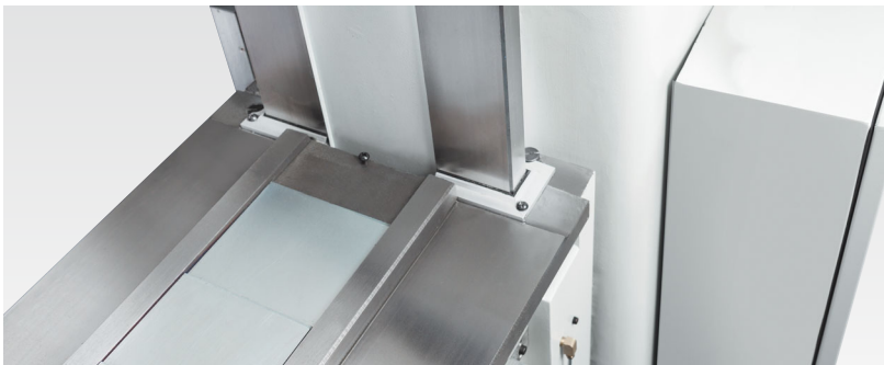
Wide, rigid box ways on Z and Y-axes
