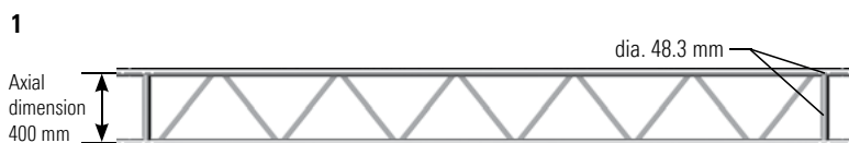
Coupler connection as in sketch possible for Ref. No. 4904
