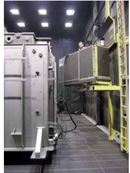
Swivelling lifting platform in a blast booth
