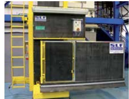
Swivelling lifting platform with wear protection for use in a blast booth
