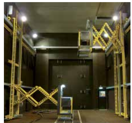
Scissor-type lifting platform in a blast booth
