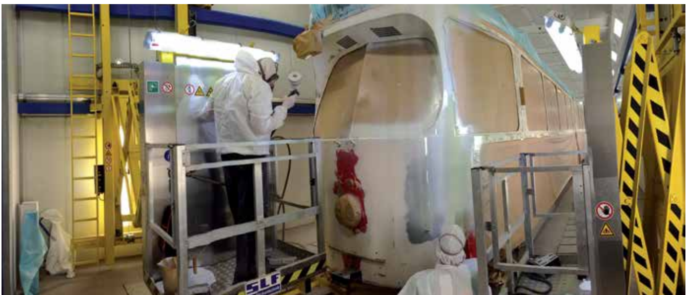
Scissor-type lifting platform in a paint-spraying and drying booth for trams
