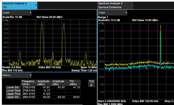
Simplify complex tasks using limit lines and built-in distortion analysis measurements.
