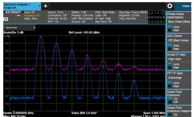
Accurately measure low-level signals to reduce measurement noise by up to 10 dB with Noise Floor Extension (NFE).
