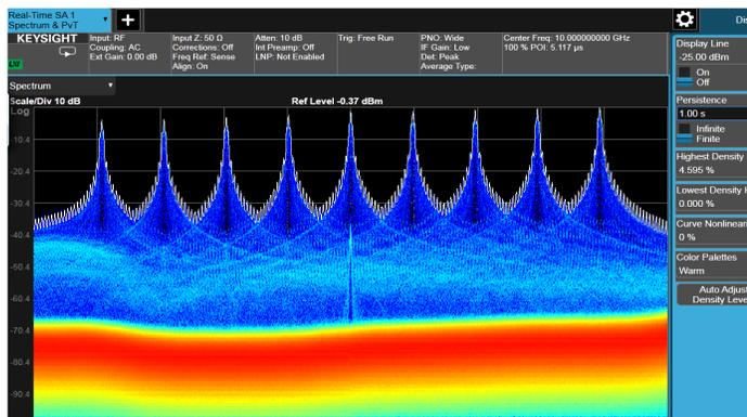
Real-time spectrum analysis bandwidth up to 255 or 510 MHz.
