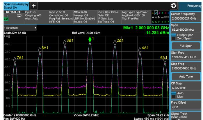
Perform essential signal characterization on signals with built-in markers and trace functions.
