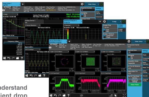
PathWave X-Series Applications allow you to see and understand the performance of your devices and designs. Convenient drop down windows enable you to quickly configure a 5G NR transmitter measurement, including 256QAM demodulation.
