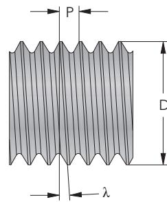
The FourCut inserts has extra clearance on the flanks and therefore it is not so important to have correct helix angle. The standard toolholder has 2° helix angle and it is possible to make almost all threads with the same holder.
