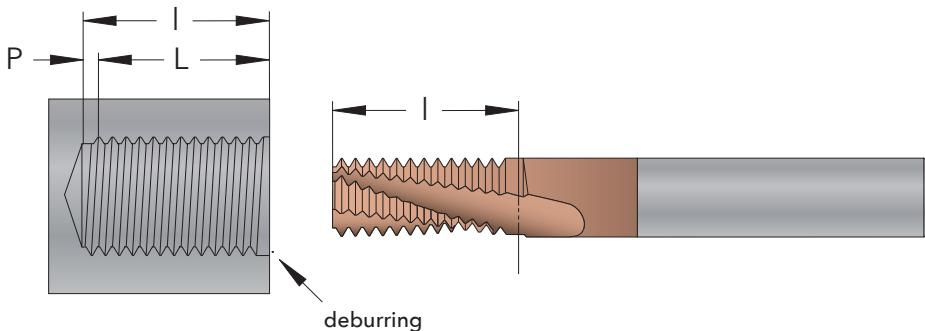
To get a nice entry and a burr free thread you need to start out with going to full depth ( $l$ ) in to the hole before starting the threading operation. The thread length ( $L$ ) will be the cutting length ( $l$ ) minus one pitch ( $P$ ).
