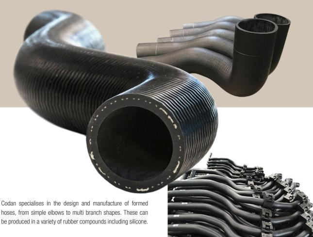
Hoses can be reinforced with heat resistant materials for pressurised systems or can be produced without any reinforcement for low pressure or vapour application. Shaped hoses can include wire support for vacuum resistance or inserted metal parts for charge points or for attachment.
