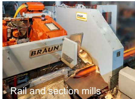
Hot rolled rails after cutting
