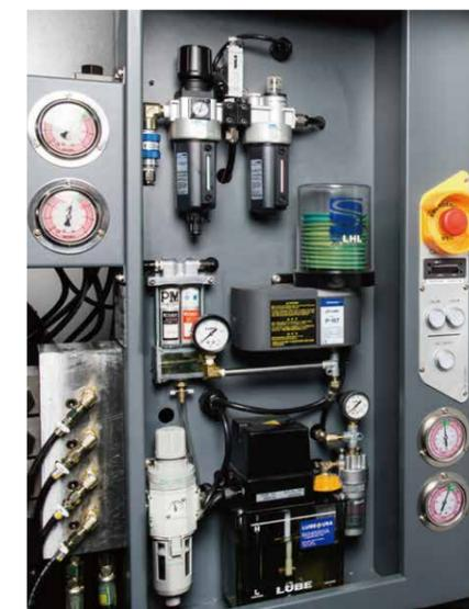
Through centralized management of air FRL unit and lubrication pump, daily maintenance becomes easier.
