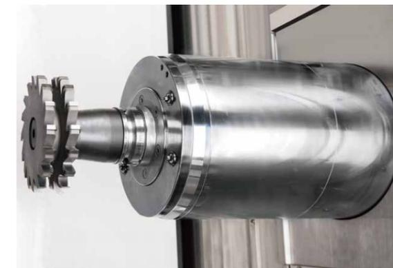
performance in aluminum alloy part, the machine is equipped with 15,000 rpm built-in spindle which has 18.5/26/37 kW power and 95/171/250 Nm torque output.
