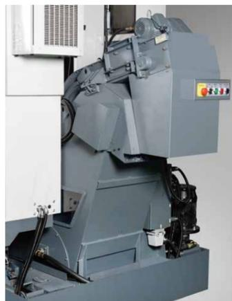
Coolant tank capacity: 700 L(80% full)
