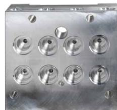
Workpiece: ABS breaking valve
