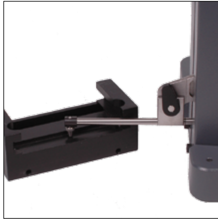
Depth measurement with accessories 930.2108 and 905.2204
