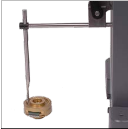
Depth measurement with accessories 930.2108 and 930.2105
