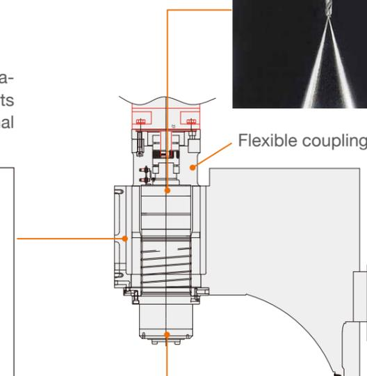
Spindle with air purge and labyrinth design avoids coolant and metal chips into the spindle.
