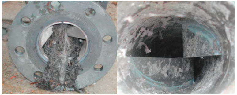
Typical clogging of competitor's mixer after less than 5 hours
