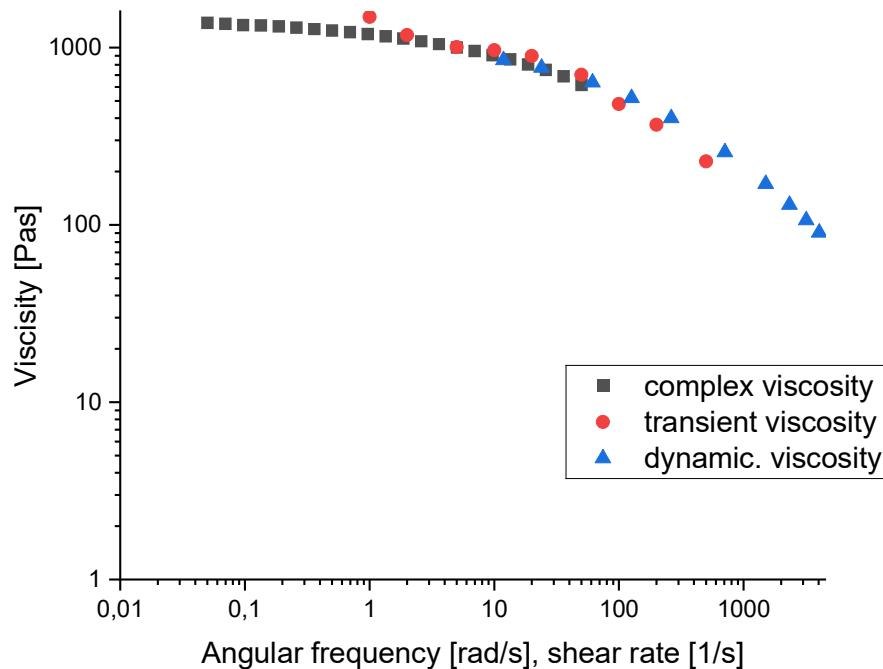
Complex viscosity: cone plate rheometer
