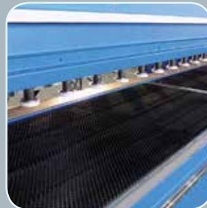
Rectangle holders with synthetic cups to cut narrow strips without being deformed
