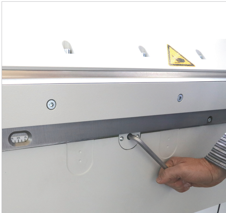
Crowning device for folding beam: manual central crowning device (not in combination with cranked folding blades)
