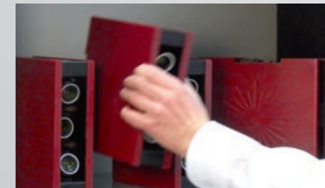
Swapping sensors is quick and easy thanks to the hot-plugging concept.
