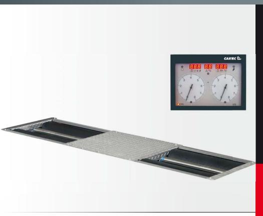
This roller brake tester is equipped with composite-coated rollers which are particularly robust. Simple operation and long life are the outstanding characteristics of this brake tester.
