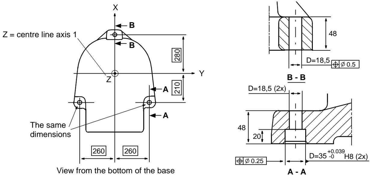
Figure 15 Hole configuration (dimensions in mm).
