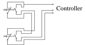
Figure 30 Connections of the switches.
