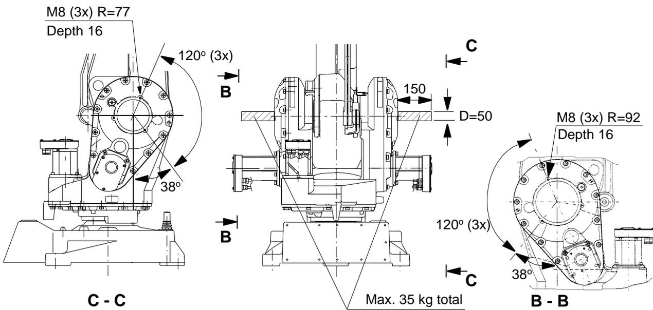
Figure 20 The shaded area indicates the permitted positions (centre of gravity) for any extra equipment mounted in the holes (dimensions in mm).
