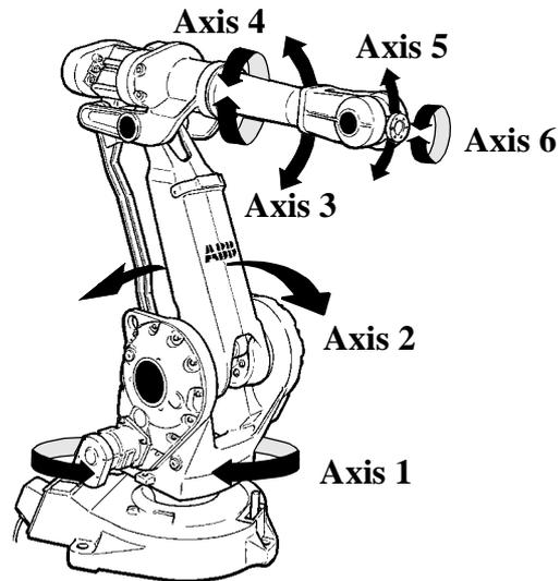
Figure 1 The IRB 2400 manipulator has 6 axes.
