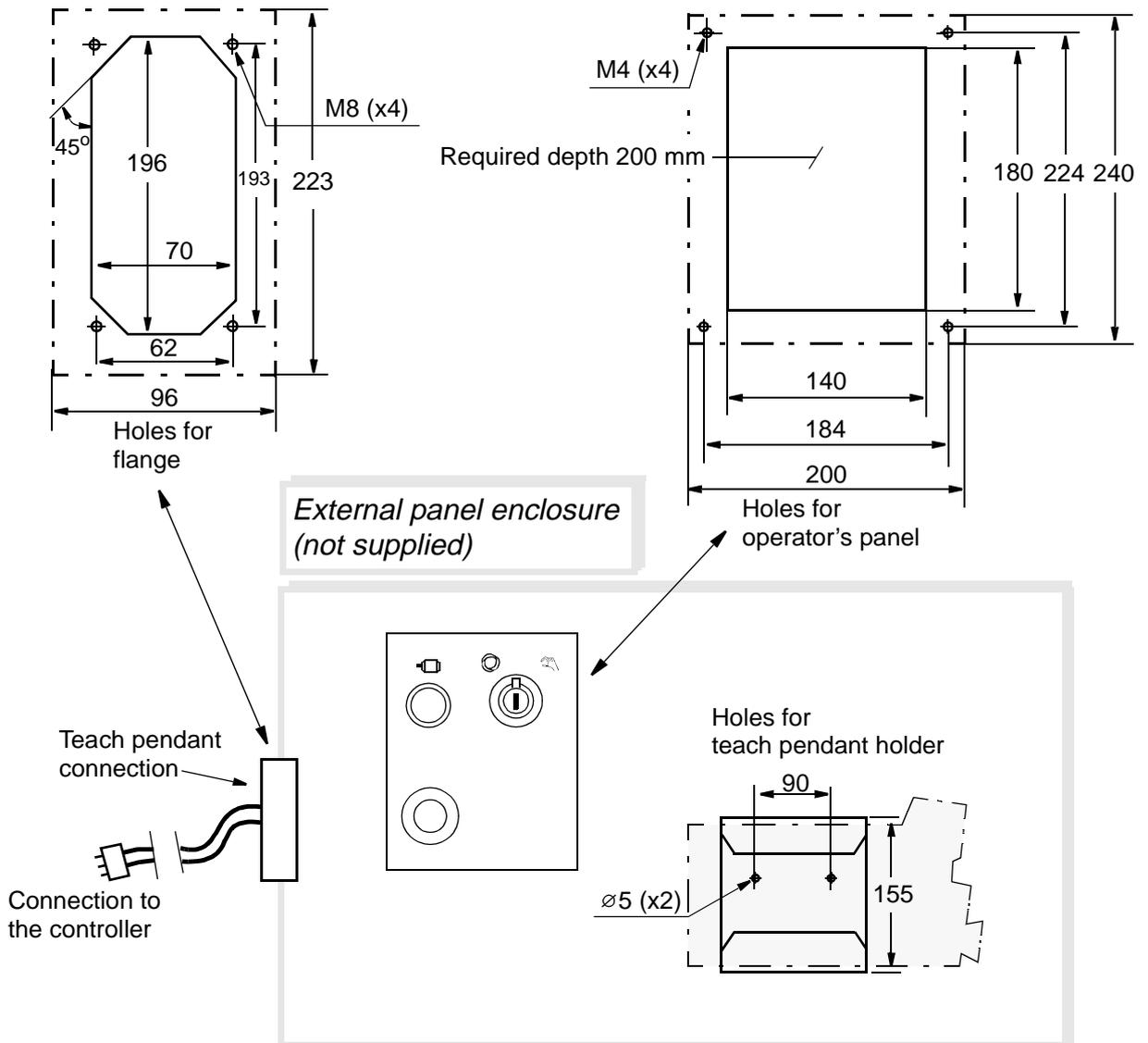
Figure 34 Required preparation of external panel enclosure (all dimensions in mm).
