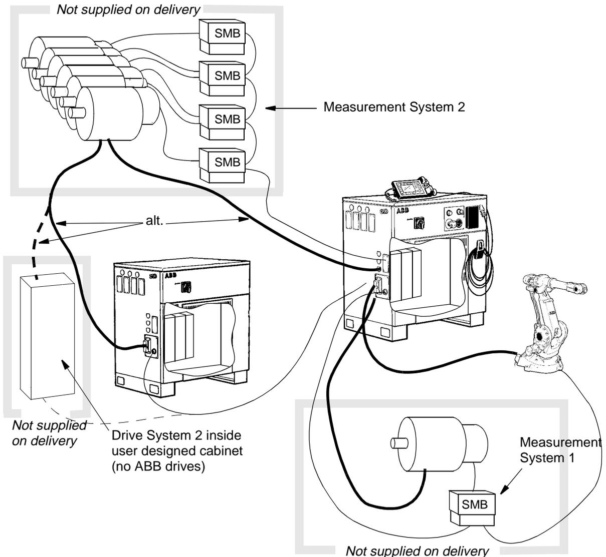
Figure 25 Outline diagram, external axes.
