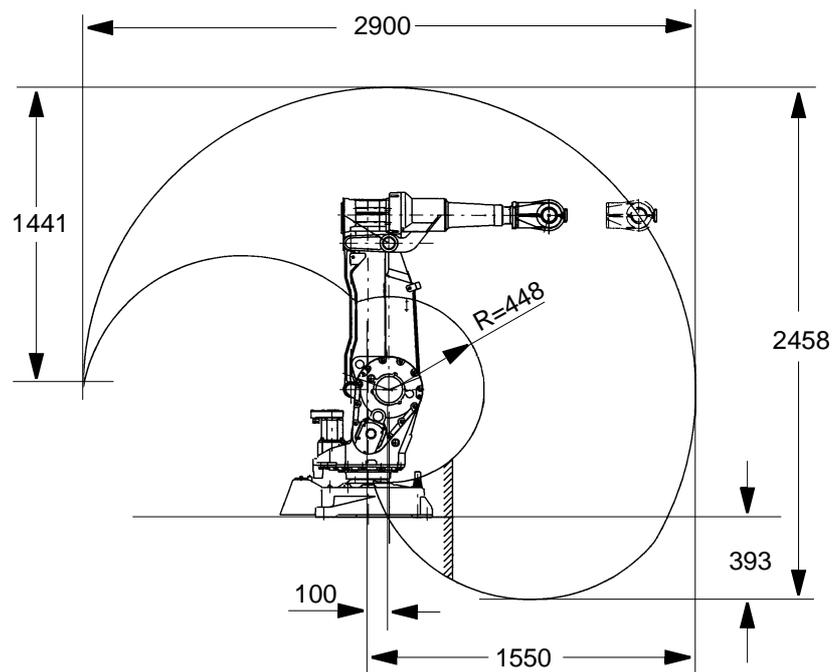
Figure 8 Working space of IRB 2400 (dimensions in mm).
