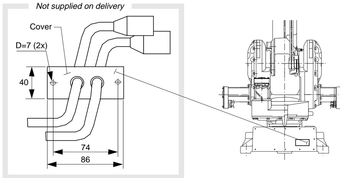
Figure 28 Cover for internal connection of signals.
