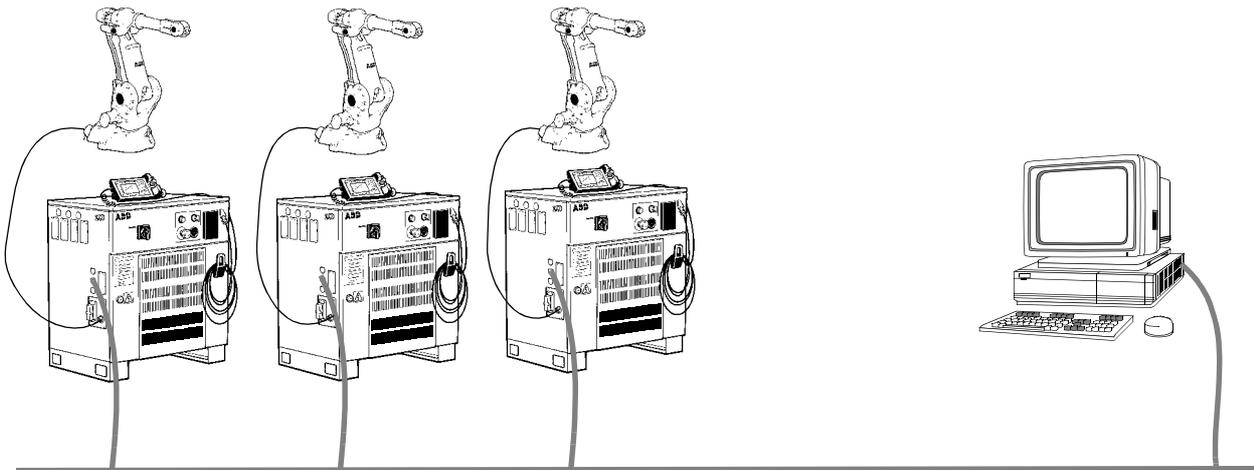
Figure 27 Serial network communication.
