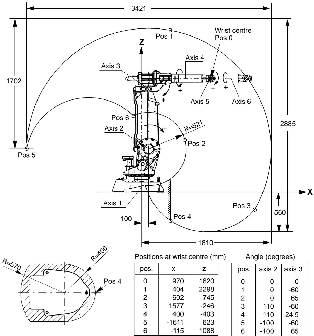
Figure 23 The extreme positions of the robot arm (dimensions in mm).
