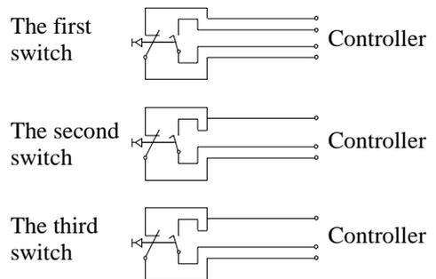
Figure 29 Connections of the switches
