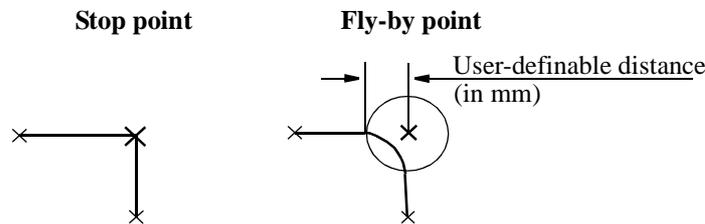
Figure 6 The fly-by point reduces the cycle time since the robot does not have to stop at the programmed point. The path is speed independent.
