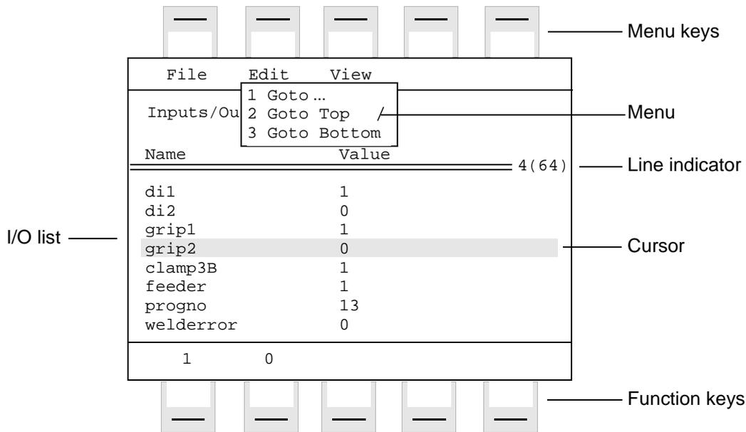
Figure 4 Window for manual operation of input and output signals.
