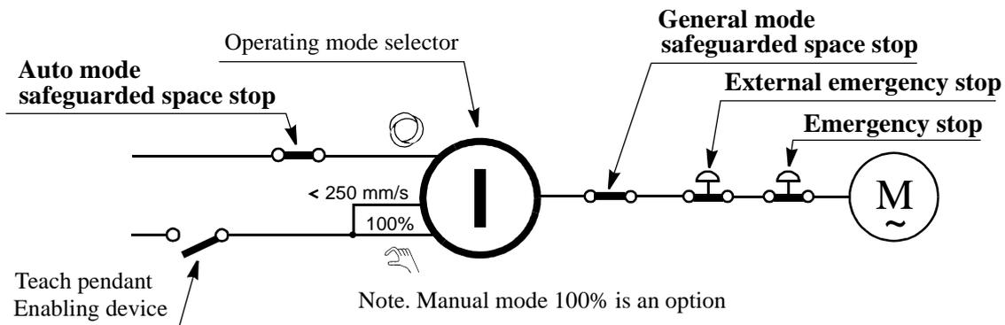
Figure 13 All safeguarded space stops force the robot's motors to the MOTORS OFF state. A time delay can be connected to any safeguarded space stop.
