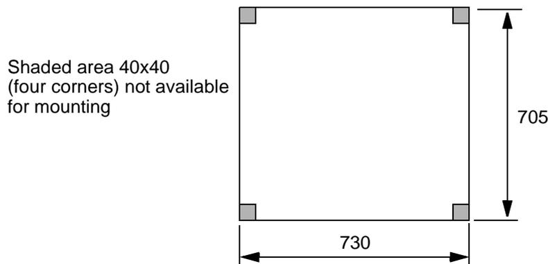
*Figure 33 Mounting plate for mounting of equipment (dimensions in mm).*
