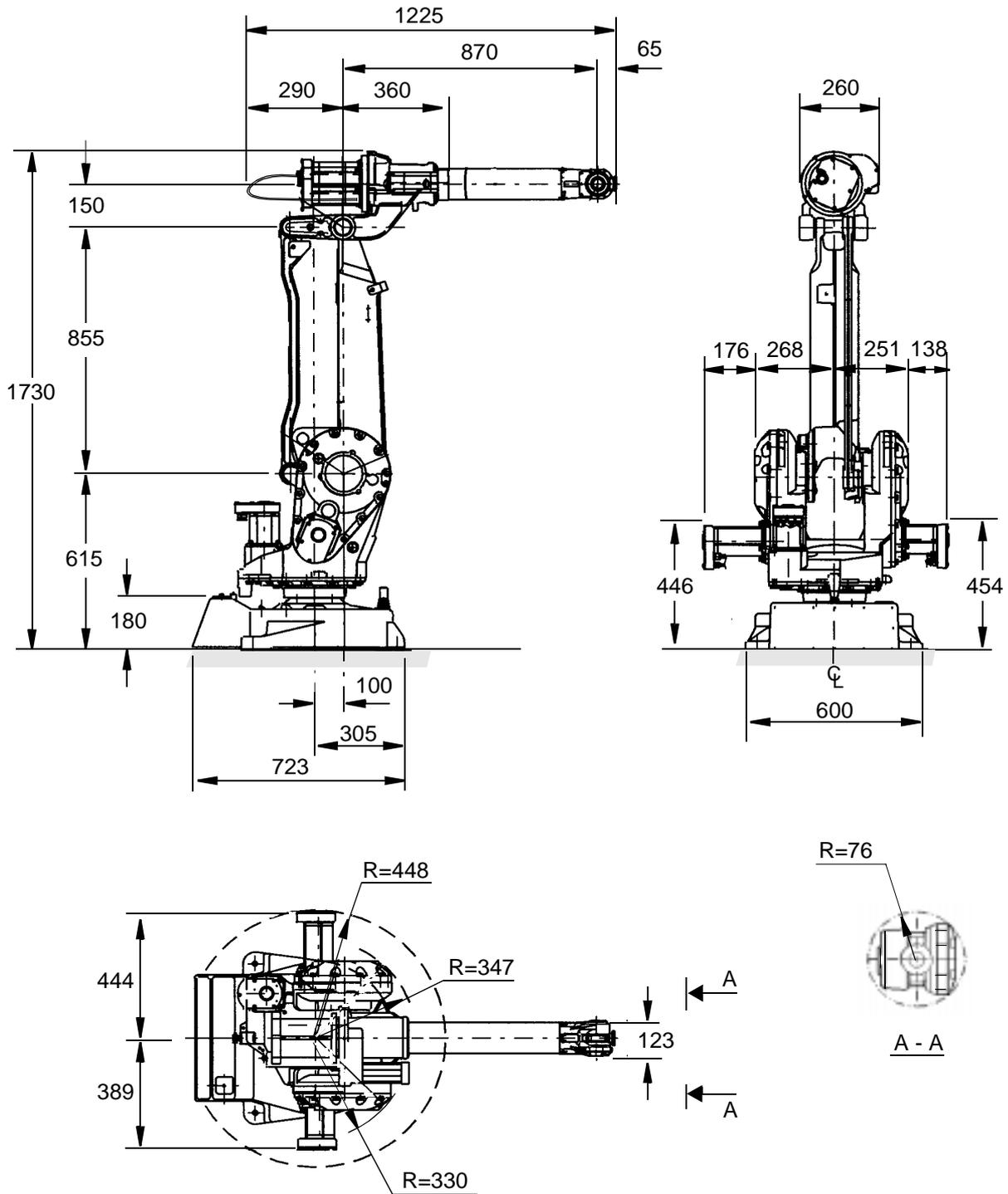
Figure 11 View of the manipulator from the side, rear and above (dimensions in mm).
