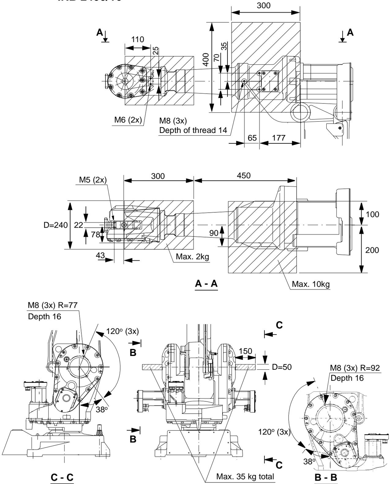
Figure 21 The shaded area indicates the permitted positions (centre of gravity) for any extra equipment mounted in the holes (dimensions in mm).
