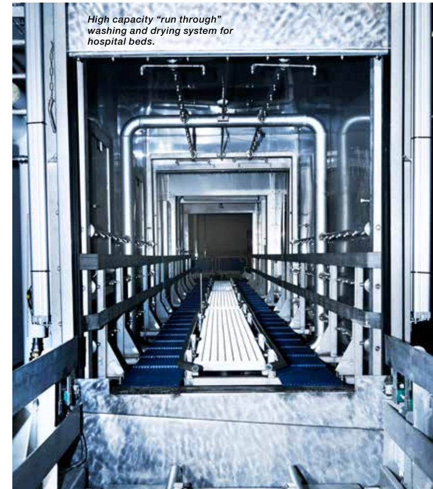
In the drying chamber the beds are dried by a set of airknives.
