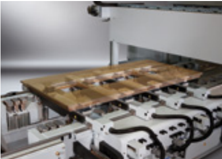
The universal clamping systems can be used simultaneously – for instance to produce front doors or semi-circular arches.
