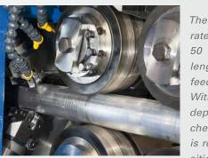
The peeling machine operates in a diameter range of 50 - 203 mm (2 - 8") with material lengths of 3 - 7 m (10 - 23 feet) and feed speeds up to 0.5 m/sec (98 fpm). With precisely controlled cutting depths of 1 - 5 mm (0.040 - 0.200 inches), the inverse segregation zone\* is reliably removed to ensure compositional uniformity through the entire cross section. Moreover, a smooth
