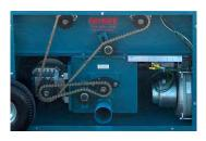
Clear Acrylic Safety Guard Allows for Inspection
