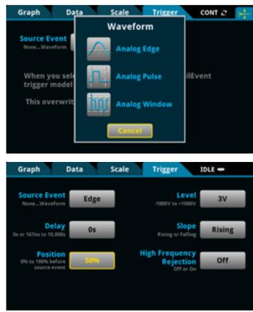
buck converter output voltage crosses the 3V trigger level, the DMM acquires the remaining 50% of readings until it returns to IDLE. **Figures 2** through **4** are a variety of power-up screen captures from the buck converter under different supply conditions. All figures contain both a trigger position indicator (▼) and a trigger level control line. You can slide this dashed line up or down to adjust the trigger level and start another acquisition.
