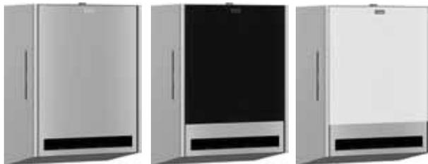
Manual paper towel roll dispenser for wall mounting, stainless steel with satin finish and InoxPlus surface refinement, material thickness 1.2 mm, max. roll width 205 mm, max. roll diameter 200 mm, paper perforation length 260 mm, adjustable paper roll holder for optimized paper dispensing, includes mounting materials. Fronts available in different versions.
