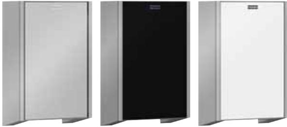
Hand dryer for wall mounting, stainless steel with satin-finish and InoxPlus surface refinement, material thickness 1.2 mm, with opto-electronic sensor for touch-free operation, adjustable hot air temperature, sensor range adjustable from 10 to 25 cm, protection from continuous operation with automatic switch-off after 60 seconds, air speed adjustable, cable and plug not included. Front cover available in different versions.
