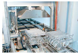
Intermediate cleaning of precision optics and ready-for-coating cleaning systems.
